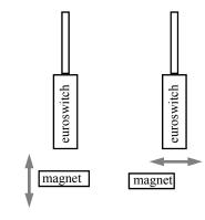
The actuator can approach the switch in two planes.
