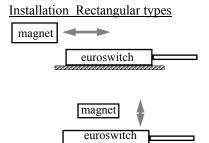
The actuator can approach the switch in two planes.
